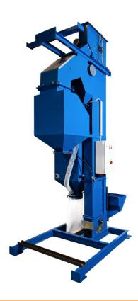
The RC50-20 is a mobile abrasive recycling machine which can be used inside or outside. Several types of reusable abrasive can be recycled by the RC50-20, the rate of recycling depends upon the type of abrasive being processed. Garnet can be recycled at a rate of up to 5 tons per hour, Steel Abrasive can be recycled at a rate of up to 12 tons per hour\*.
